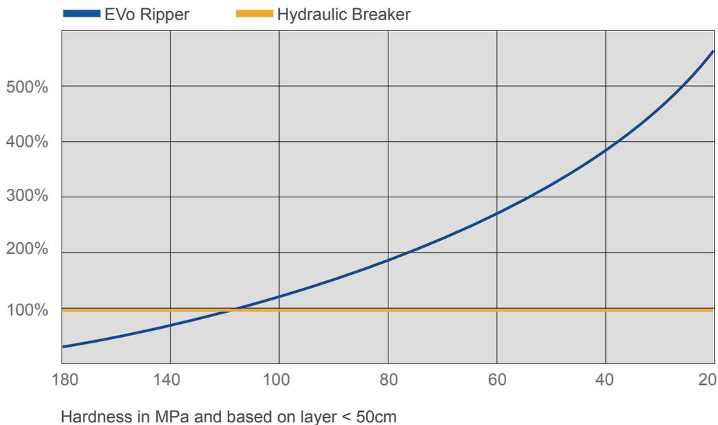
The Evo Ripper combines the working principles of impact force of a hydraulic breaker with vibration and ripping power of a conventional ripper. Due to this combination of both breaking, vibration and ripping, it can produce up to five-times higher excavation rates compared to conventional hydraulic rock breakers.
